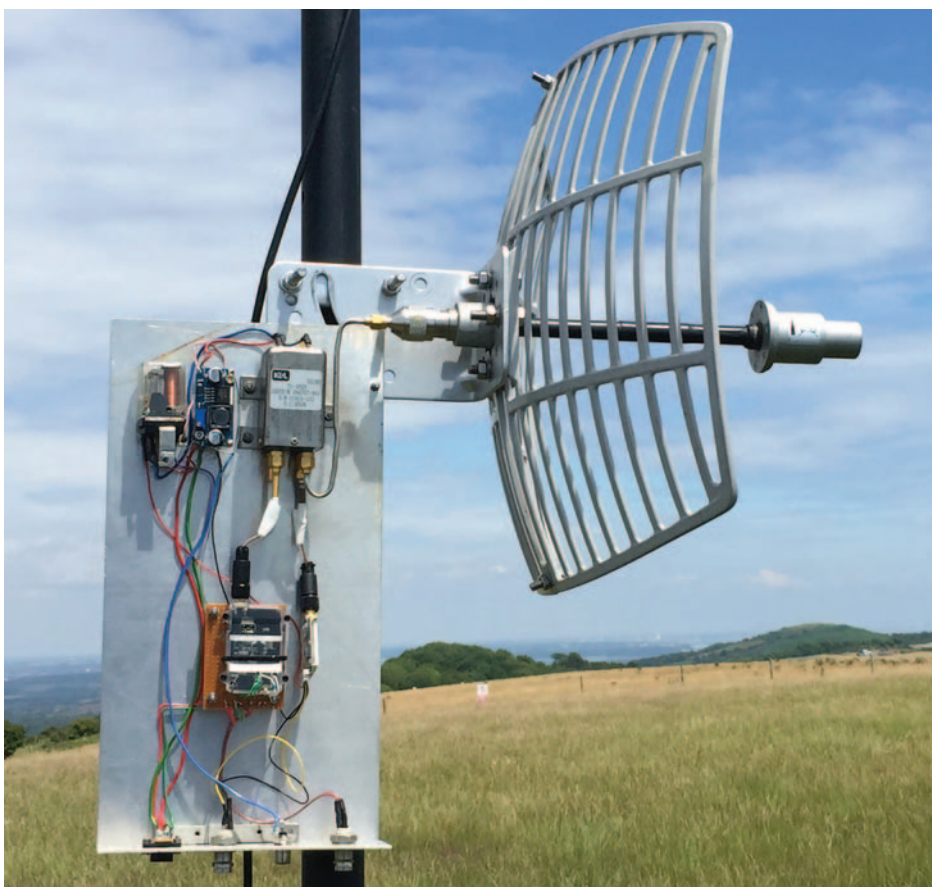
PHOTO 1: 6cm FM ATV transceiver setup.
