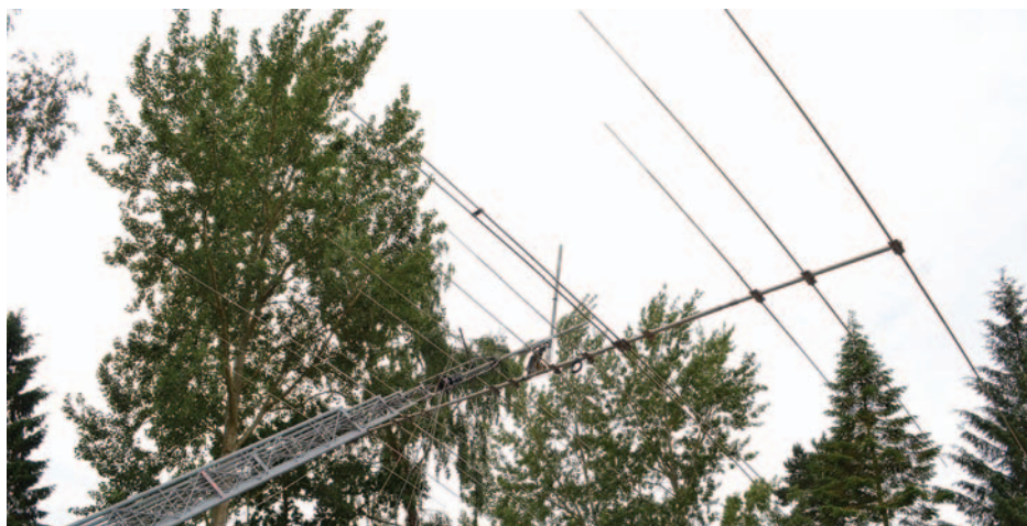
The boom truss with the supporting cable can be seen near the centre.
