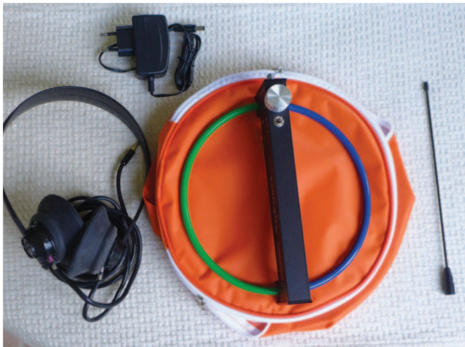
PHOTO 1: The FoxRex 3500 is pictured on top of the orange carrying case. The robust pair of headphones are on the left, the E field whip on the right and the (EU plug) mains power supply is at the top. The manual is not pictured.
