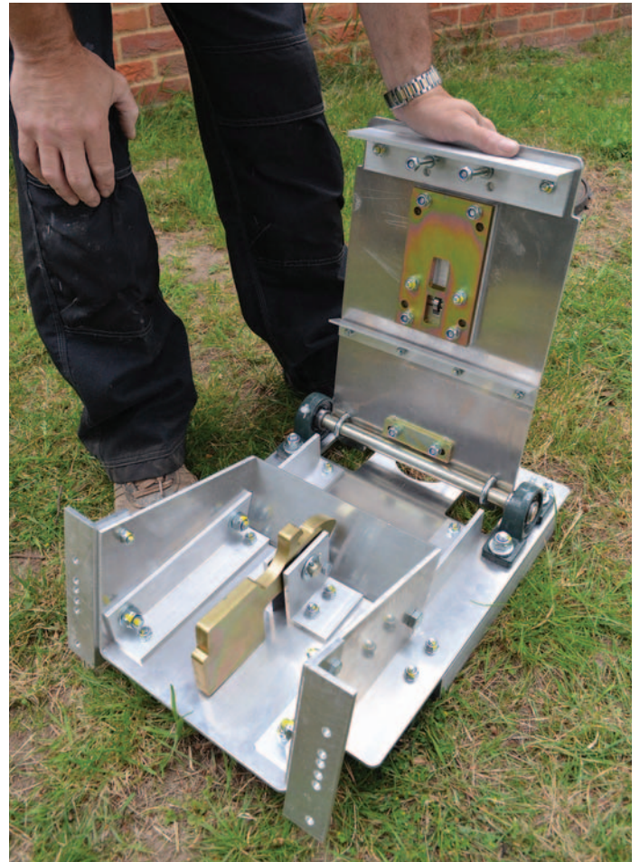
This shows the pendulum assembly (centre) that locks the plate into position.
