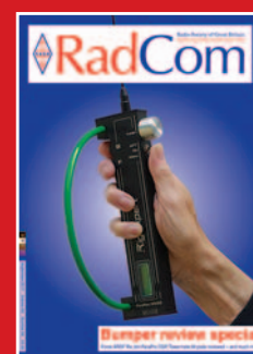
Cover image: The FoxRex 3500 80m amateur radio direction finding (ARDF) receiver. Image by Bob Titterington, G3ORY.
