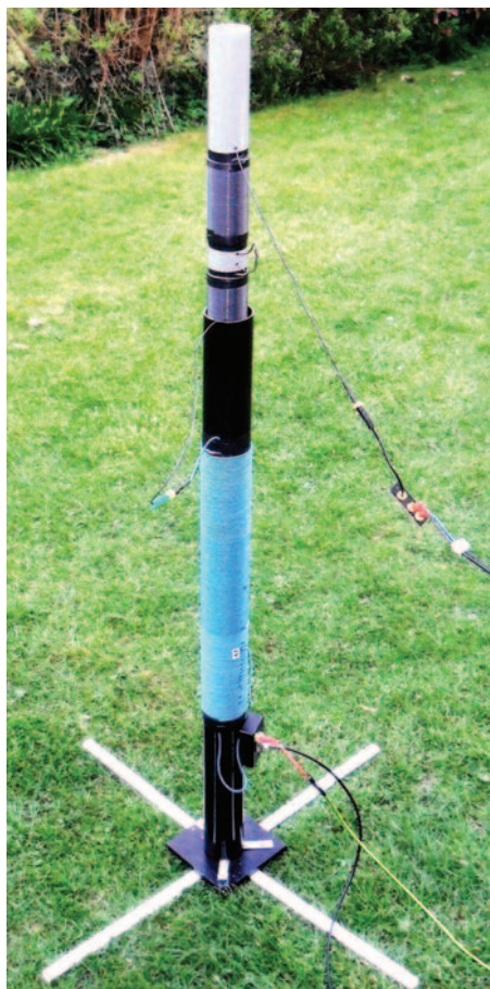
PHOTO 1: The auto-transformer/variometer antenna matching system used for operation on 630m.
