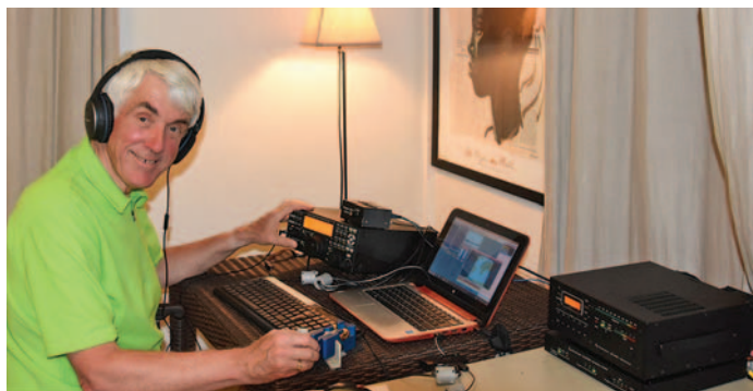
3B8/G3TXF with Elecraft K3S, KPA-500 amplifier and KAT-500 ATU. Logging with Win-Test ("...still the best!"). (Photo courtesy of G3TXF).
